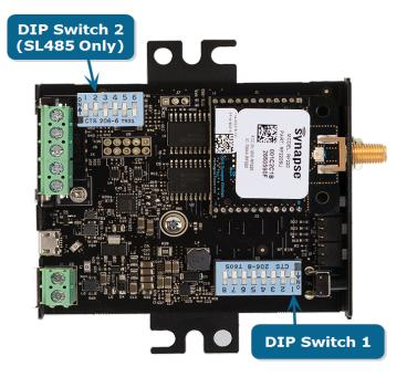
To access the DIP switches, remove the screw adjacent to the serial connection (DE-9 connector or terminal block) and lift the top of the enclosure off to expose the switches.
