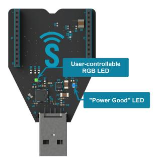
The SN132 was designed to primarily act as a bridge device. The only user-accessible GPIO is connected to the multi-color LED, controlled by SNAP GPIOs D1, D2, and D3.
