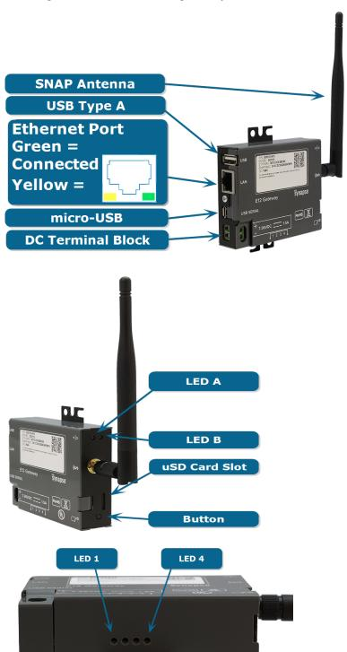
All E12s include a SNAP-powered module, and will come with an antenna for the module's connection labeled with the Synapse S on the E12's case.
