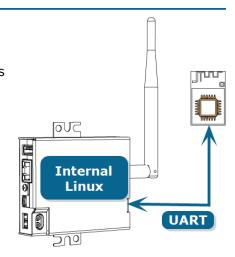
In addition to the serial connections, there is one GPIO pin from the E12 that is tied to the module for controlling and signaling.
