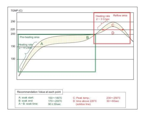
Figure 1.7: Reflow Profile Graph
