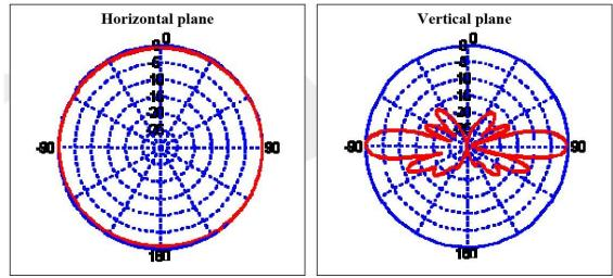
Figure 1.6: ANT-OSC-8.0-1 Antenna Gains Performance
