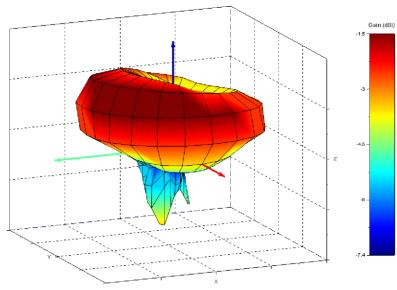
3D Radiation Pattern - Total Gain at 2370 MHz
