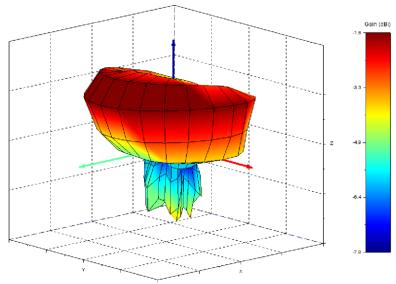
3D Radiation Pattern - Total Gain at 2440 MHz
