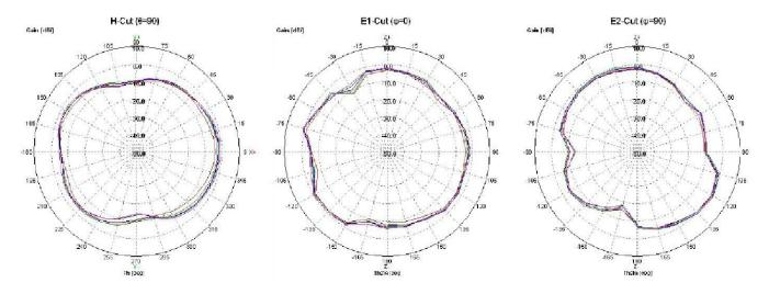
Figure 1.5: ANT-2.4-CW-RAH-RPS Antenna Gains Performance
