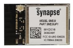
also includes a Skyworks SE2431Lfront-endmodule, which provides a power amplifier and LNA for increased range.
